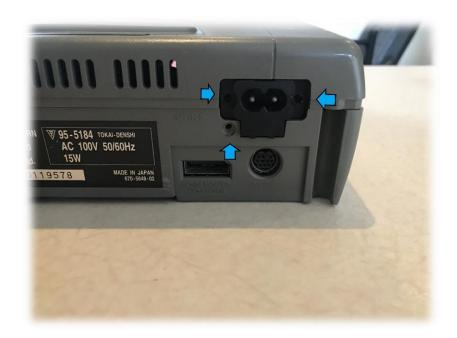
3- Remove the top lid of your console, unscrew the stock PSU (it can be either attached to the top shell for the VA0 revision or to the console chassis for the VA1-15), and unplug all cables. **Remove the PSU**.
