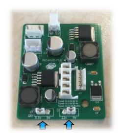
For **Type A**: Set jumper S1 to 3.3v and S2 to 9v
