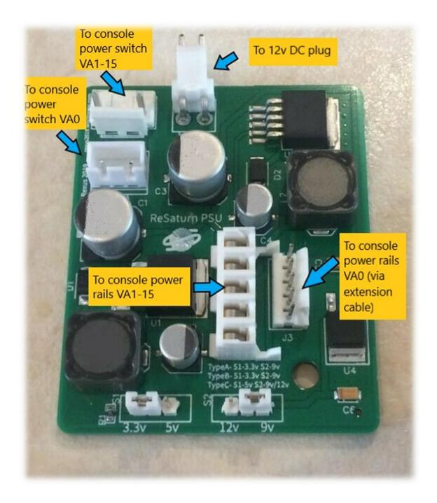
11- The **ReSaturn PSU** has a hole on the PCB to fix it on the chassis with the original screw. However, there are some chassis revisions that have this hole positioned in a slightly different way. If your revision does not align with the **ReSaturn PSU**, cover the small flap on the metal chassis with some electric tape. Just to make sure you don't have any short:
