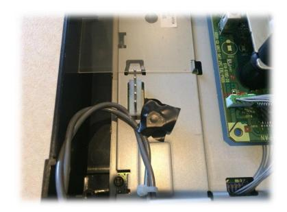
12-If you have a VA1-15 revision, just plug the PSU into the rails, screw the DC socket at the back using the two screws from the original PSU and you're good to go:
