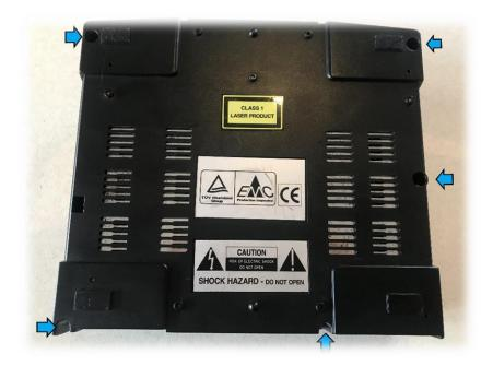
2- Unscrew the two/three screws that hold the original PSU together with the console shell (where the 110v or 220v- plug is connected).
