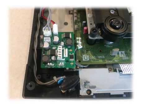
13-If you have a VAO, use the four bits of double sided tape (included) to attach the **ReSaturn PSU** on top of the plastic that isolates the stock PSU from the metal chassis (the **ReSaturn PSU** should sit on top of it as per the picture below). Above all, make sure there's no contact between the back of the PSU and the metal chassis.
